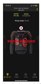
Figure 18: Tech-Air® App System view when no more Gas Inflators (17) are available
